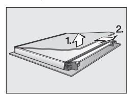
■ **Gently** lift the inner pane up and pull out of the cover strip.
